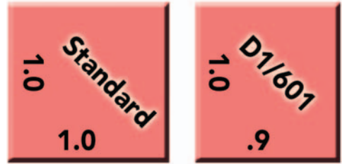
A standard square and NTSC D1 pixel.
