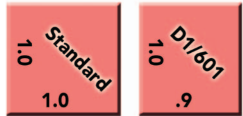
A standard square and NTSC D1 pixel.
